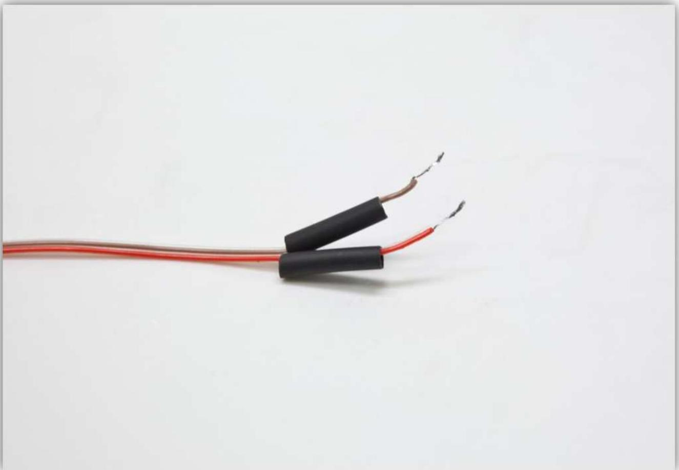
Solder the wires to the contact points of the micro switch, slide the heat shrink tubes over the contacts and shrink them.
