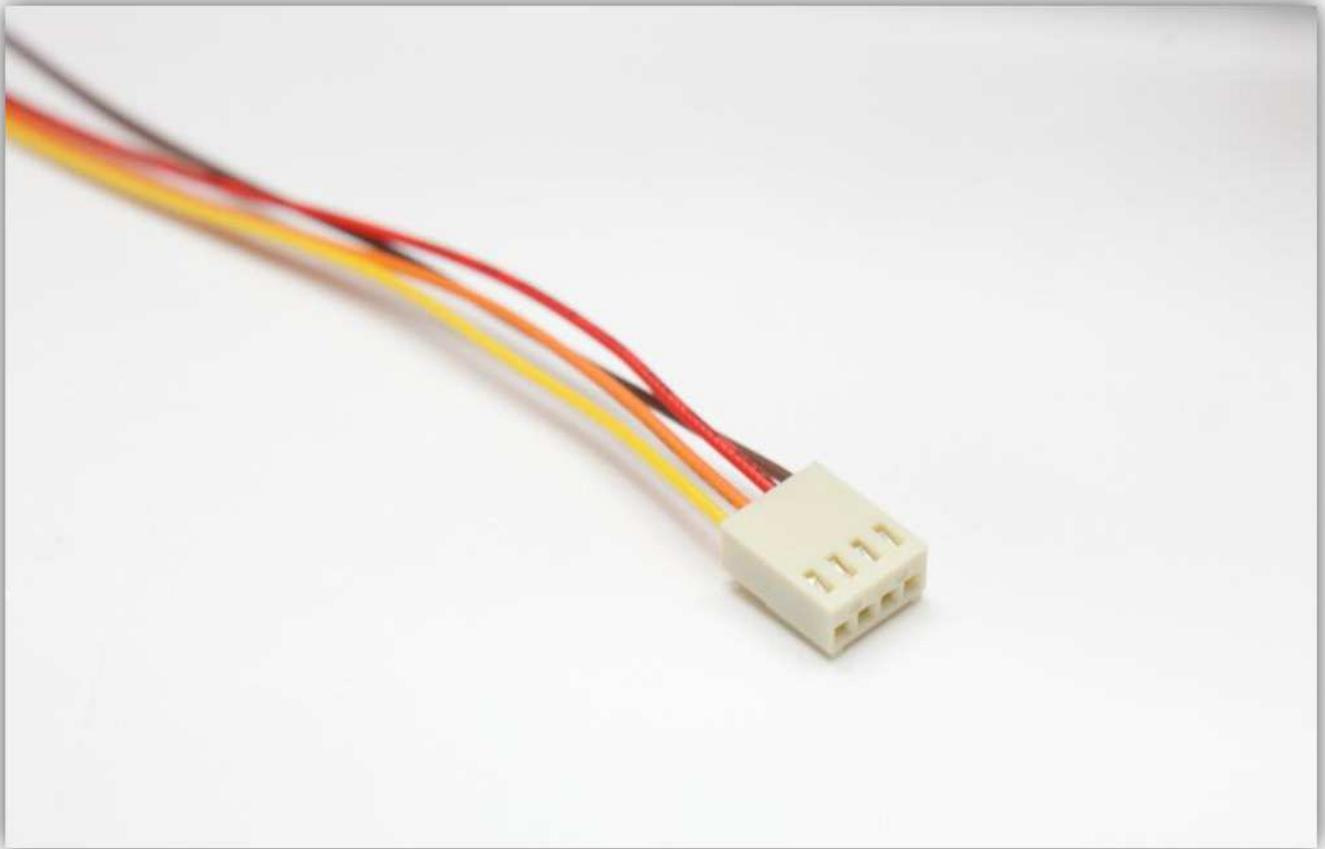
Plug the female connector in the male connector labelled with X-MOTOR on the controller board.
