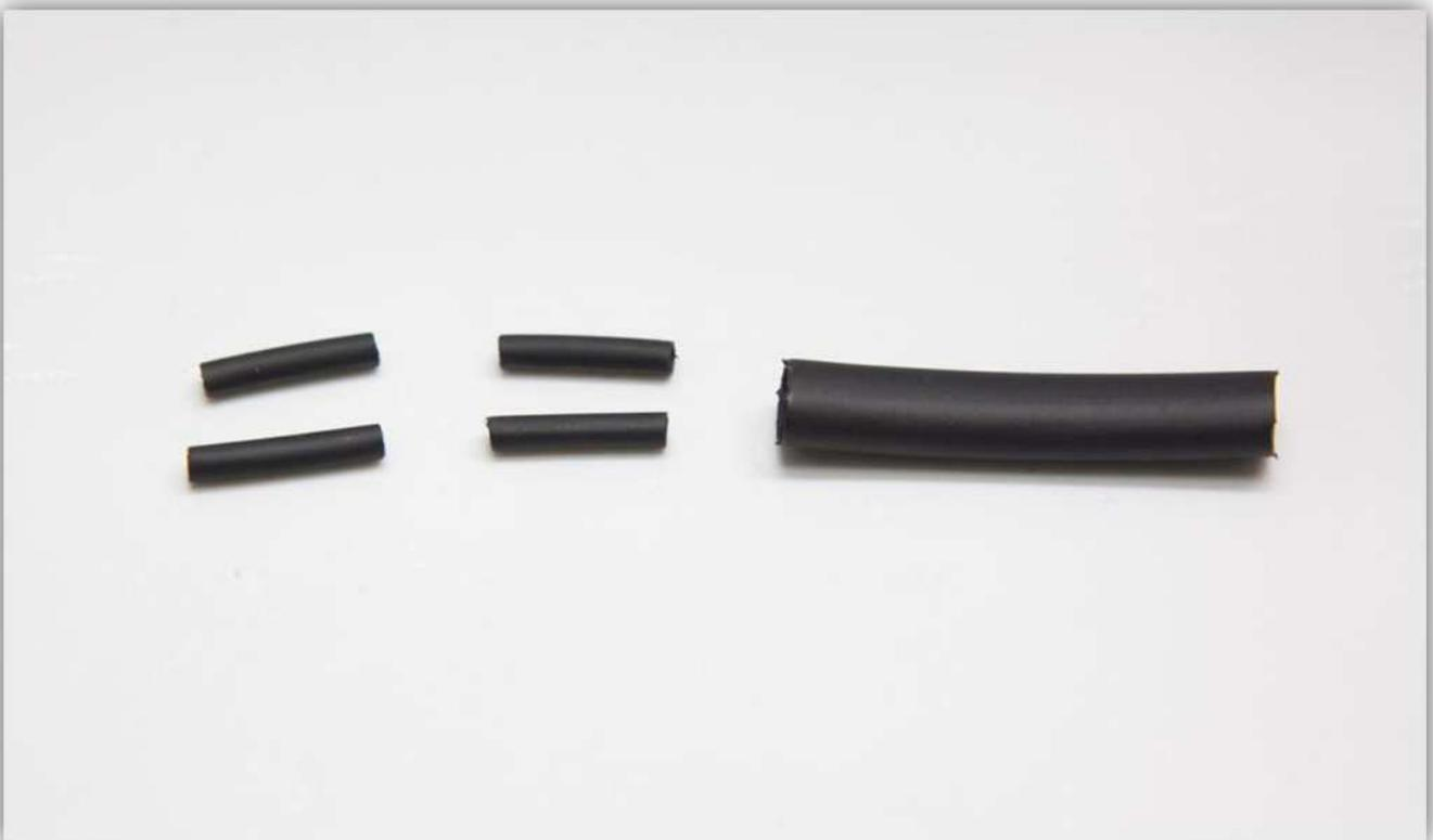
Slide the big heat shrink tube over the 4 wires of the connector.
