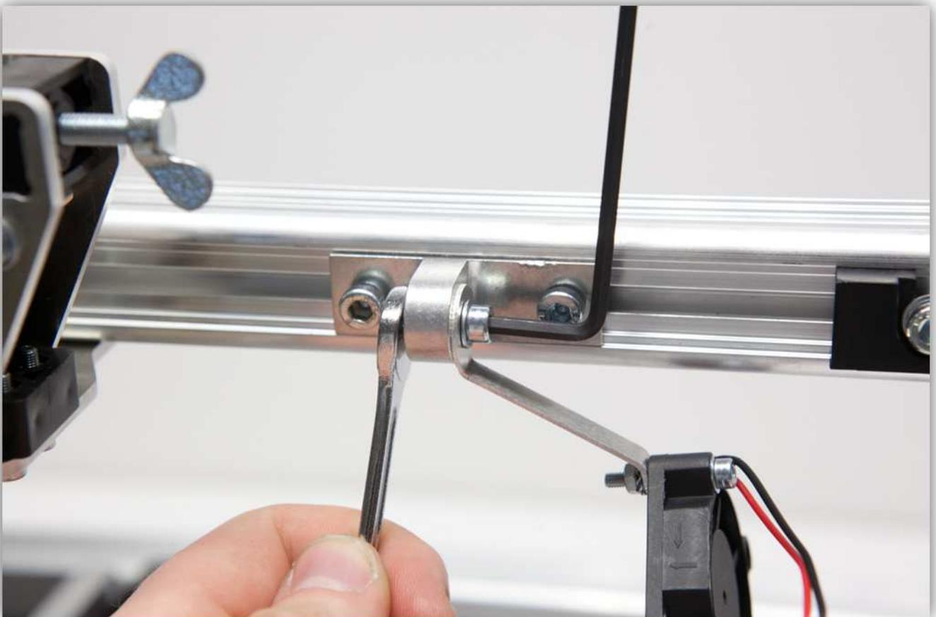
Tighten the bolt on the fan, make sure that the fan is level.
