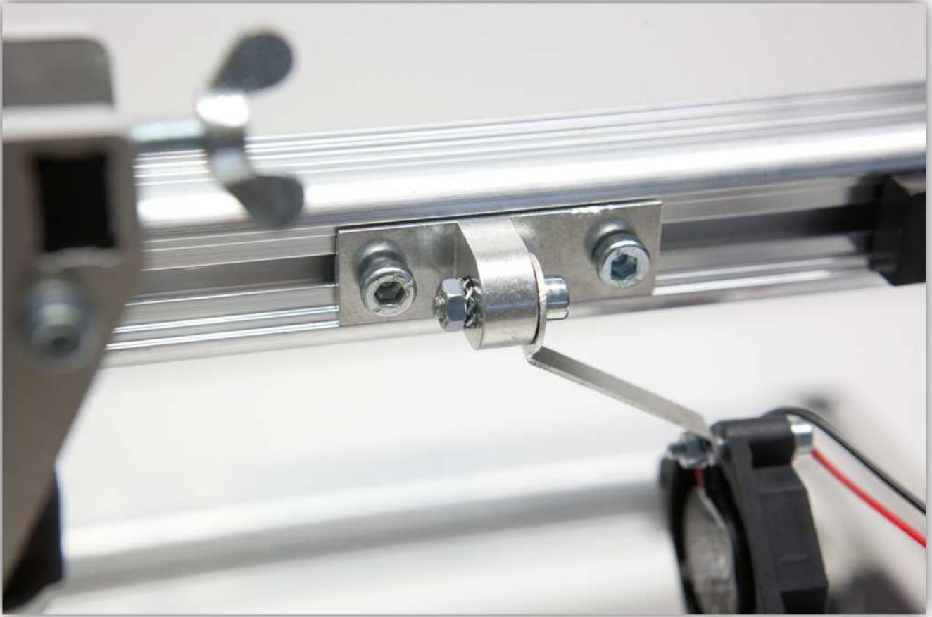
Tighten this bolt, make sure that the FAN HOLDER is vertical.
