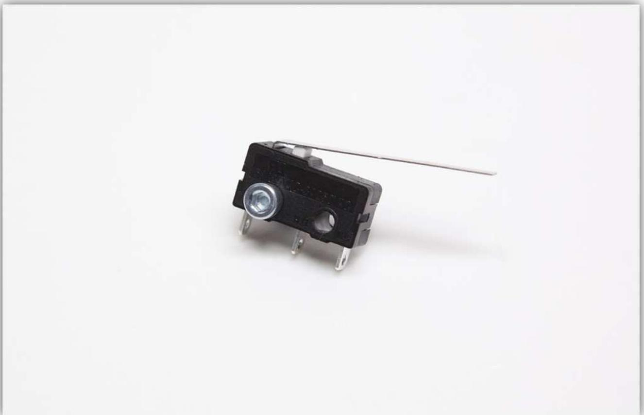
Bolt the micro switch to the Z MOTOR BRACKET, use an M3 bolt. **Make sure it is level.**
