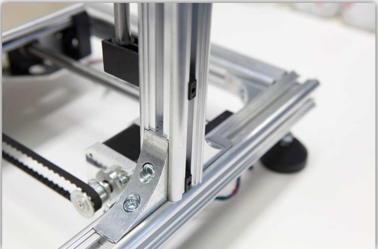
Next slide the COIL SUPPORT in the same profile and align it with the horizontal ALUMINIUM PROFILE. Tighten it firmly.
