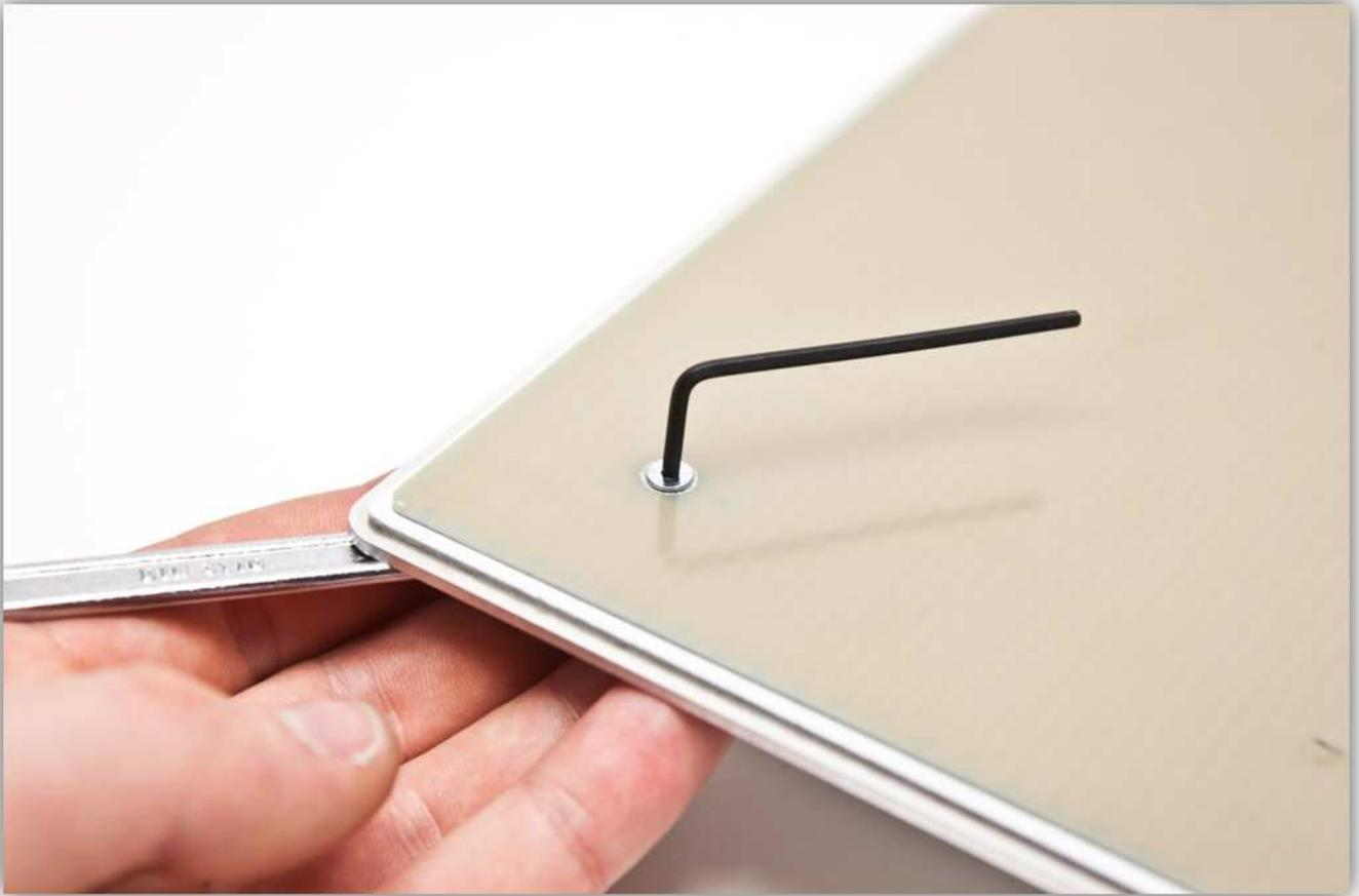
Insert an M4 nut into 4 THUMB SCREWS.
