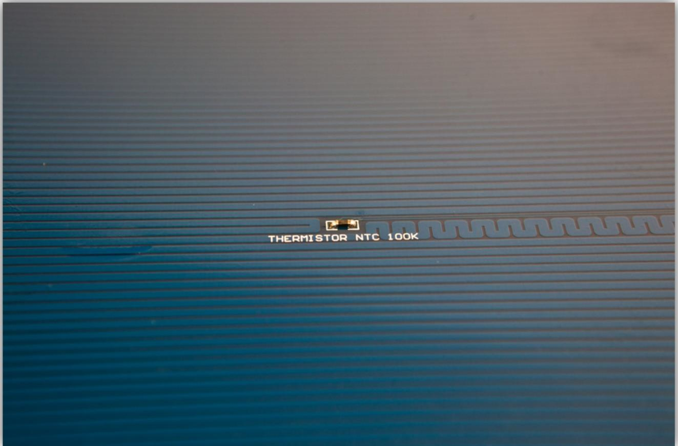
Place the HEATED BED PCB on the BED PLATE. **Watch the orientation carefully.**
