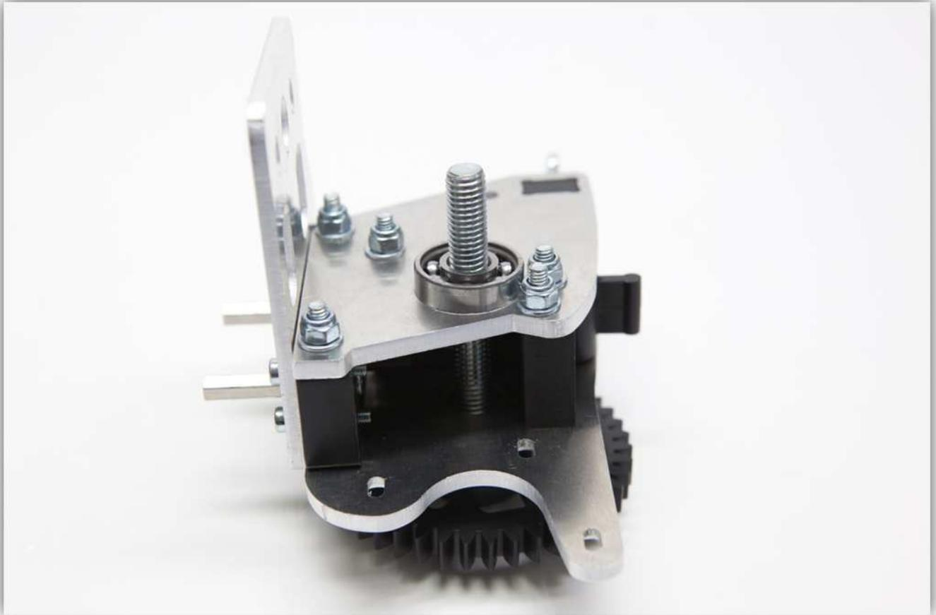
Slide an M8 washer to cover the 608 BEARING.
