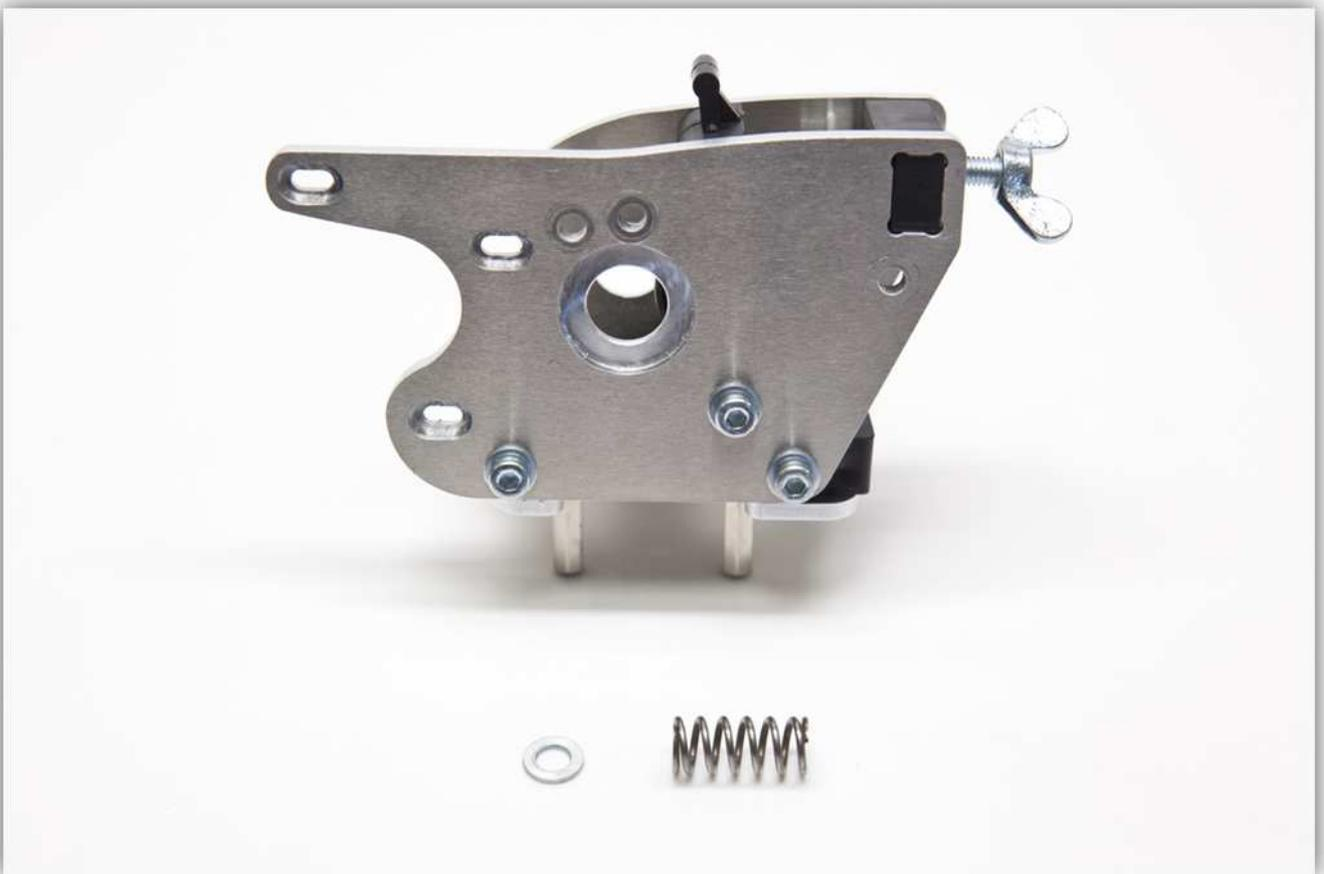
Place the spring into the cavity of the BEARING CLAMP assembly.
