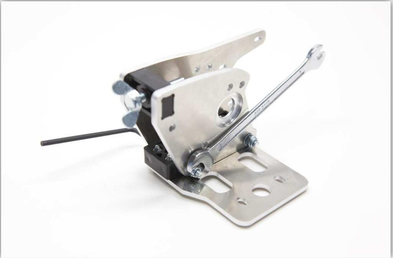
Tighten the bolts that hold the EXTRUDER MOUNT PLATE to THE EXTRUDER BASE.
