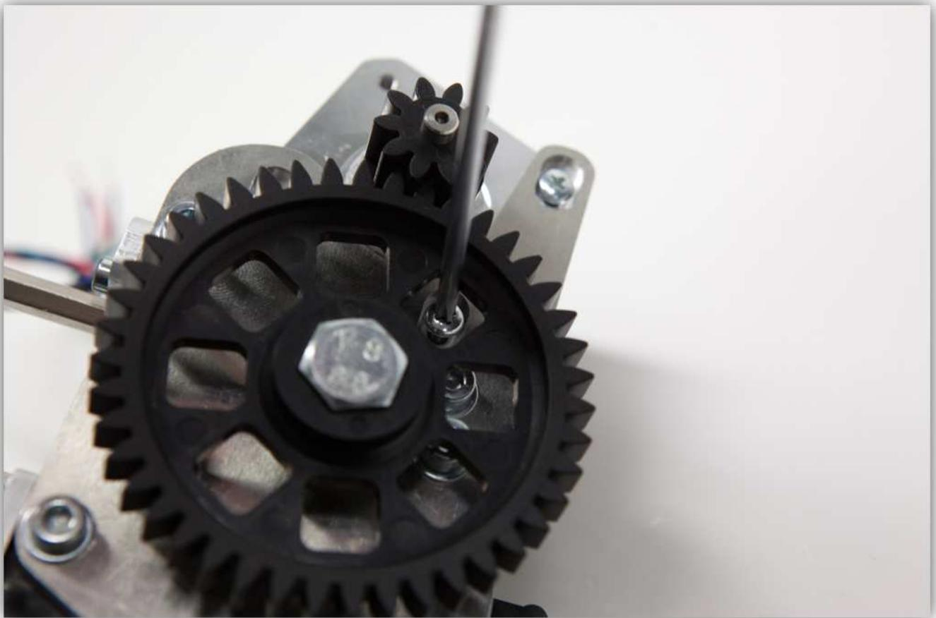
Position the motor so the teeth of the gears interlock as shown in the picture below. **Then you can fully tighten the bolts.**
