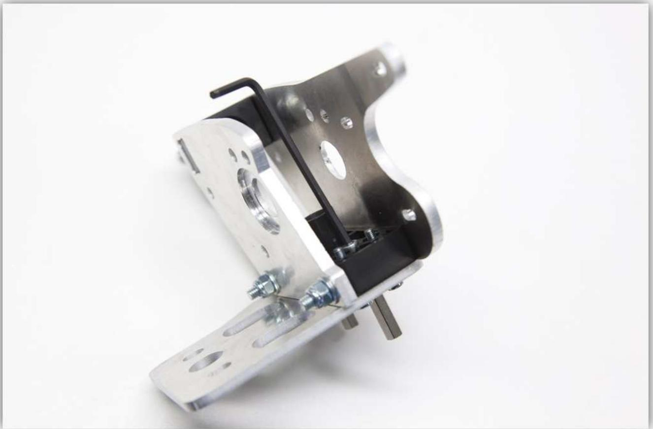
Slide the BEARING CLAMP assembly into the extruder assembly.
