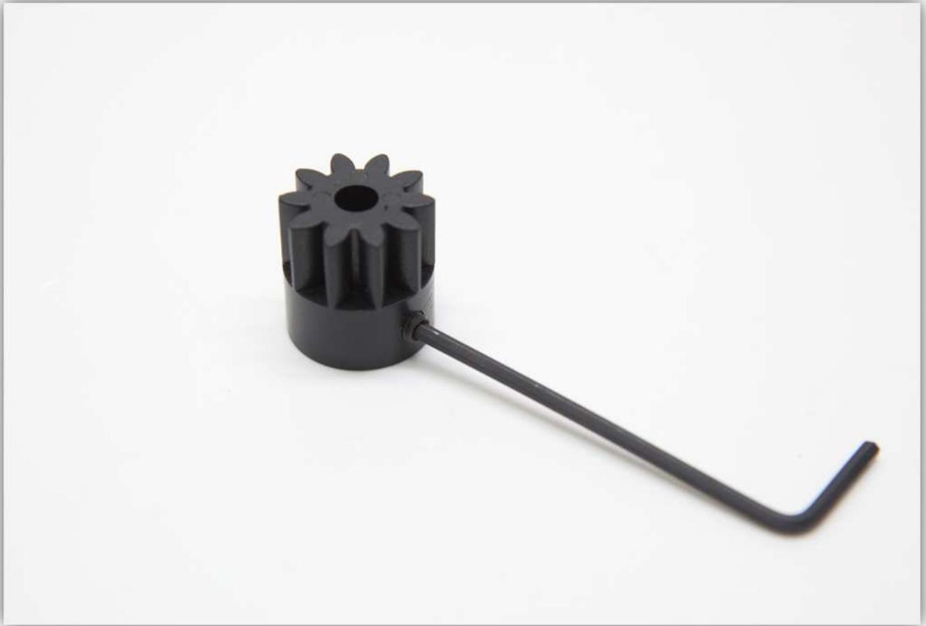
Now take a motor out of the package labelled with 9 and slide the small gear over the shaft. **Slide it down until there is just place for a piece of paper between the motor and the small gear.** Then tighten the small locking bolt.
