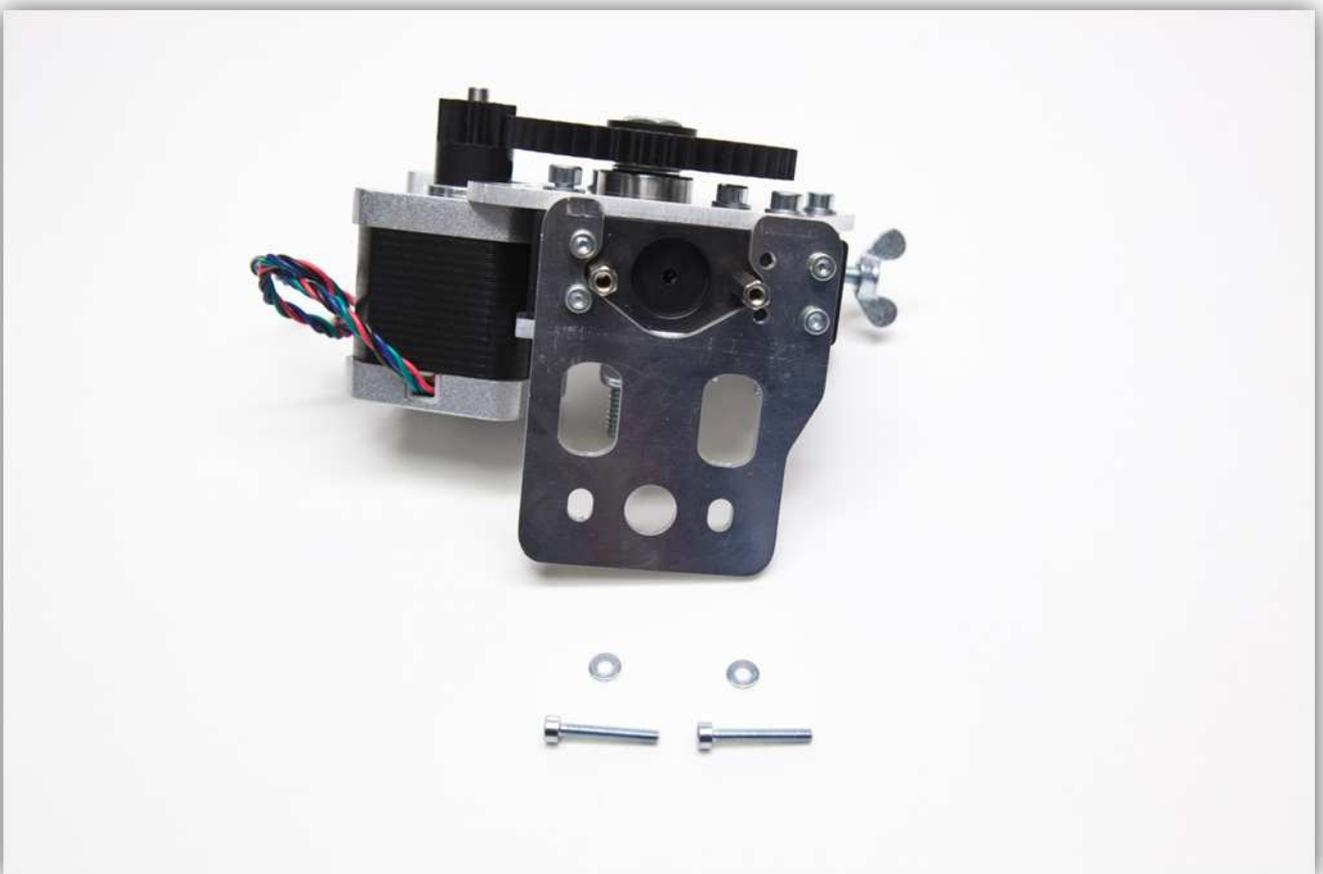
Screw these into the spacers for later use (the extruder itself will be mounted with these bolts.)
