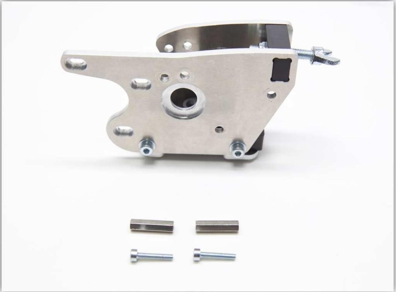
Slide the two bolts into the EXTRUDER BASE piece as shown in the picture below.
