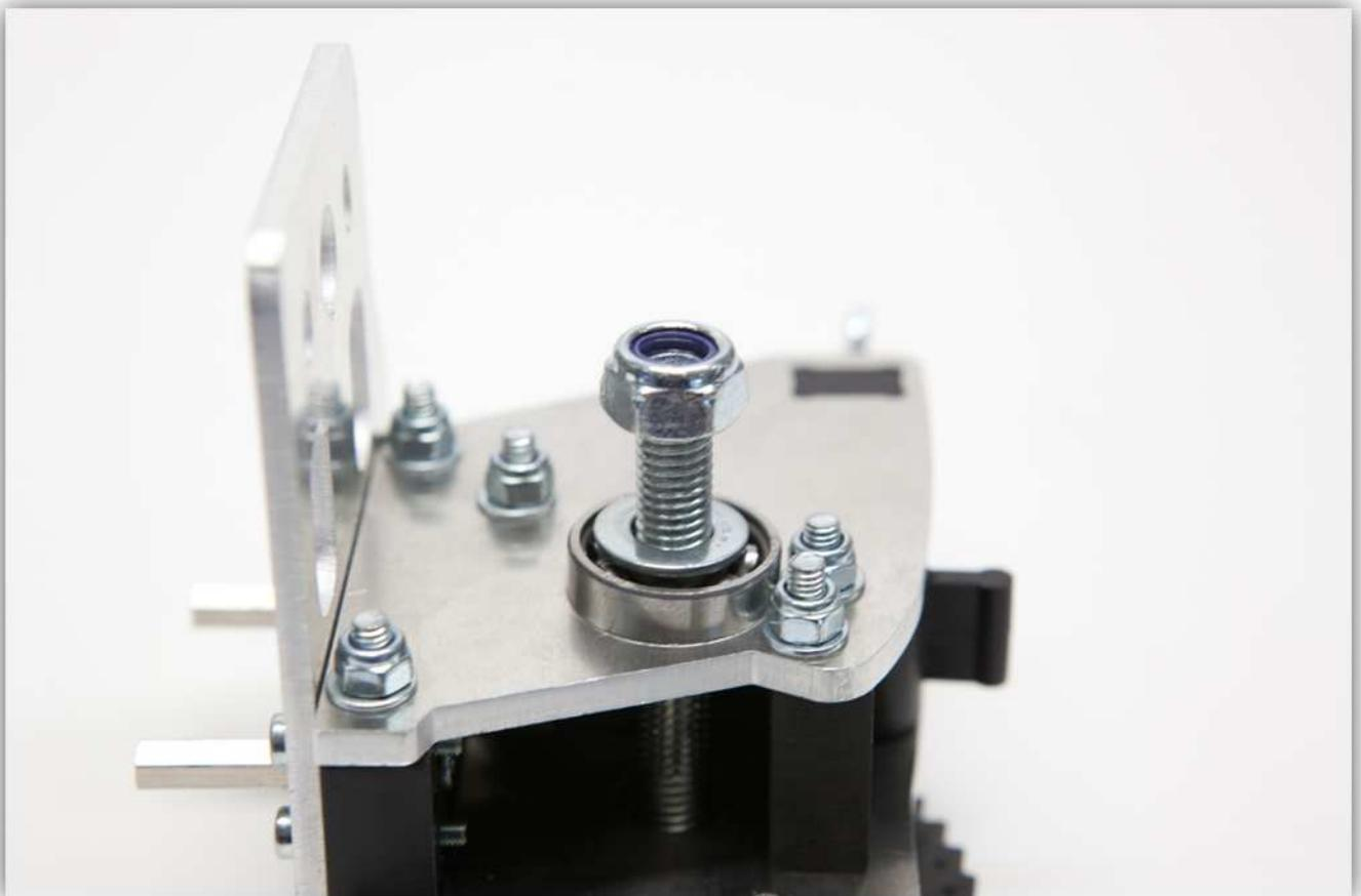
Tighten this bolt but make sure that the large gear turns smoothly.
