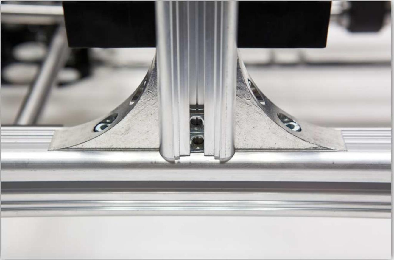
Use 2 M5 bolts and 2 M5 toothed washers to bolt the Z MOTOR BRACKET to the frame.
