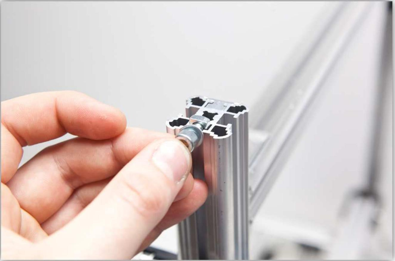
Slide the assembly over the Z ROD GUIDE and tighten the bolt so that it is fixed but still possible to slide up and down.
