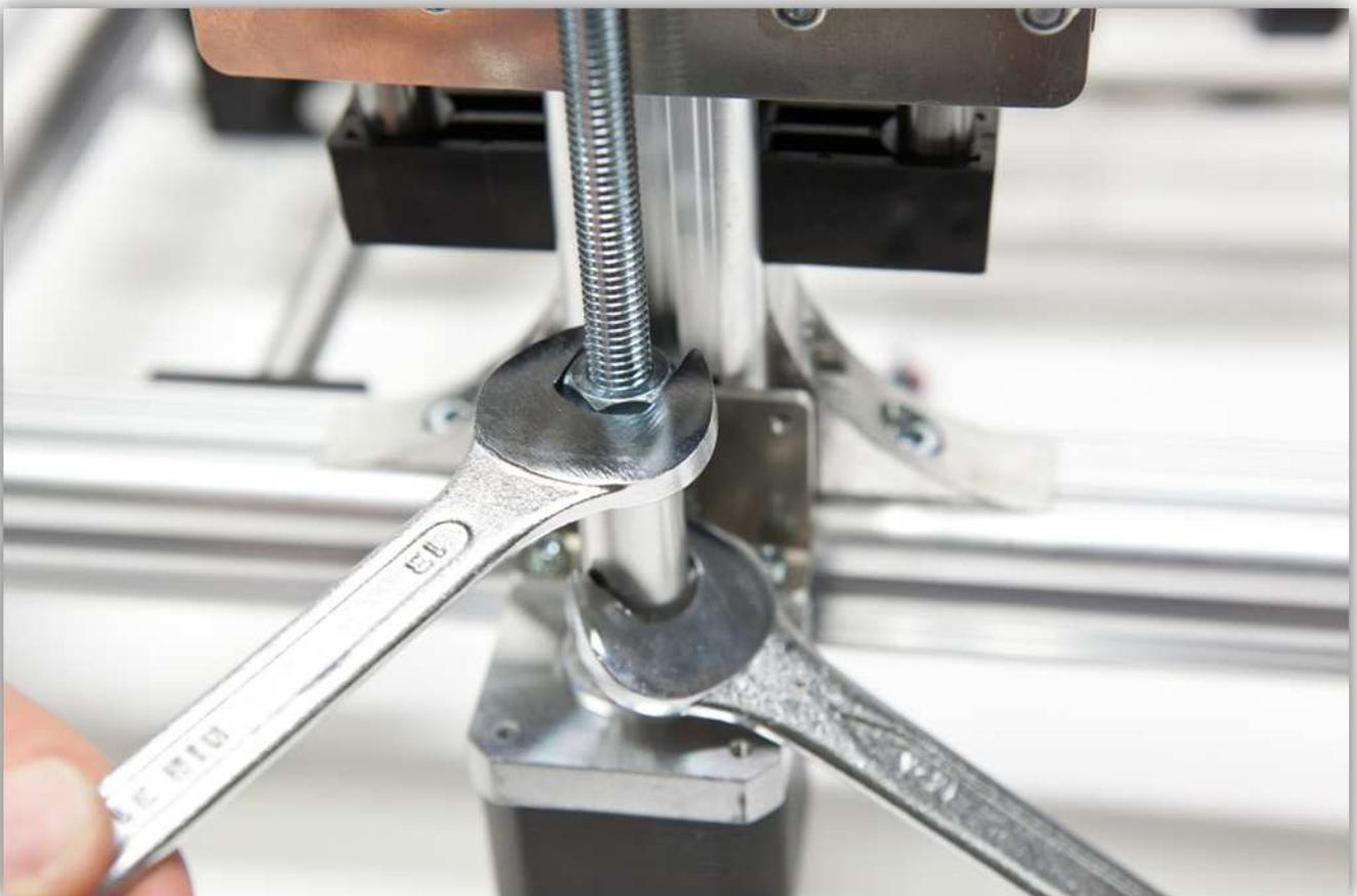
Attach the Z FOLLOWER A piece to the CARRIAGE. **Do not fully tighten these bolts.** Turn the rod until the M8 bolt sits snugly into the Z FOLLOWER A piece.
