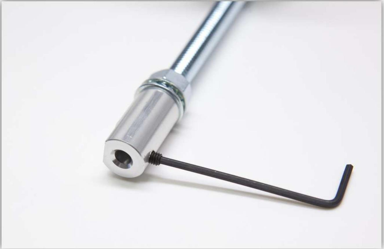
Place the MOTOR CONNECTOR over the motor shaft. Make sure that the shaft goes as far as it can. Now tighten the small locking bolt.
