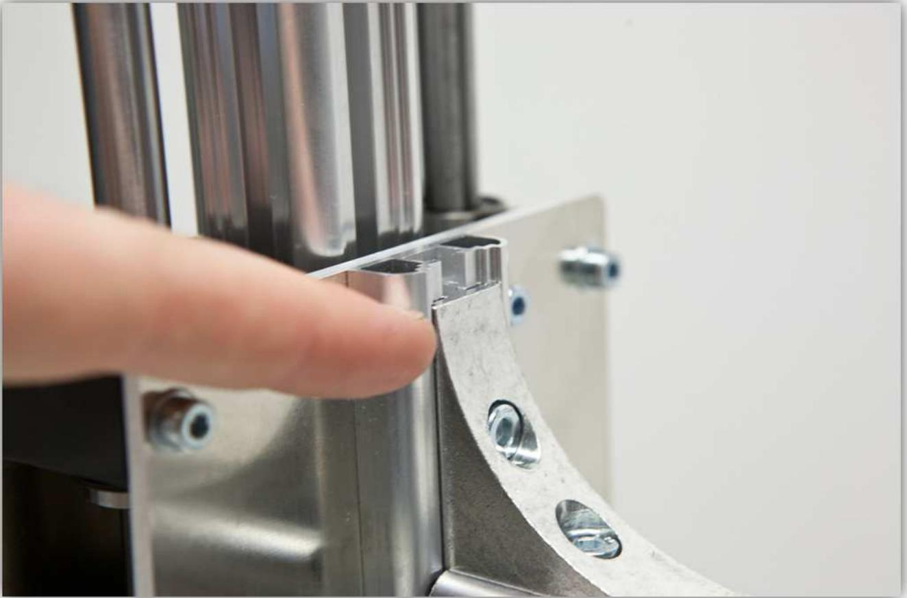
Tighten all the bolts on the ANGULAR MOUNTS.
