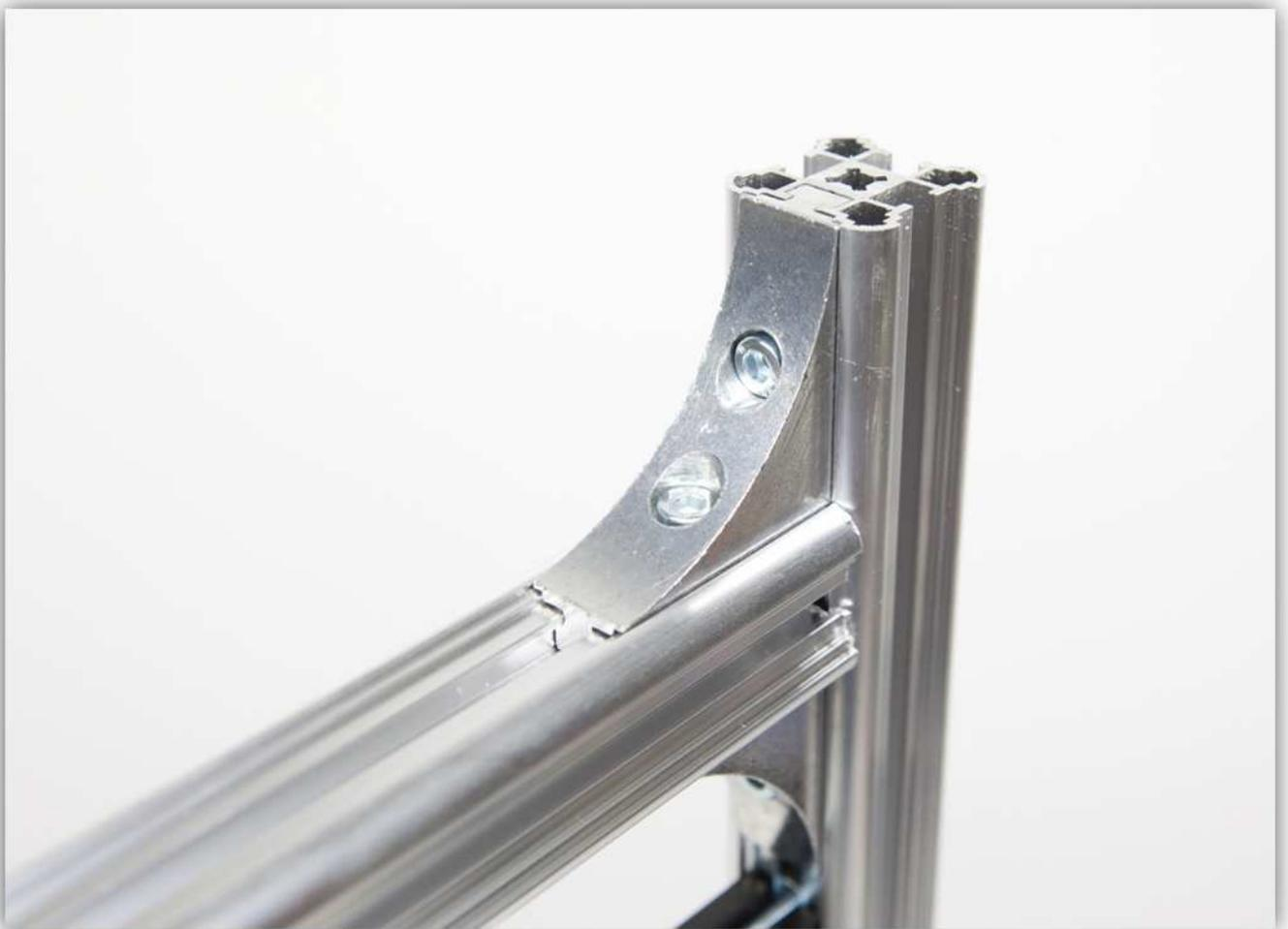
Tighten all the bolts on the angular mounts.
