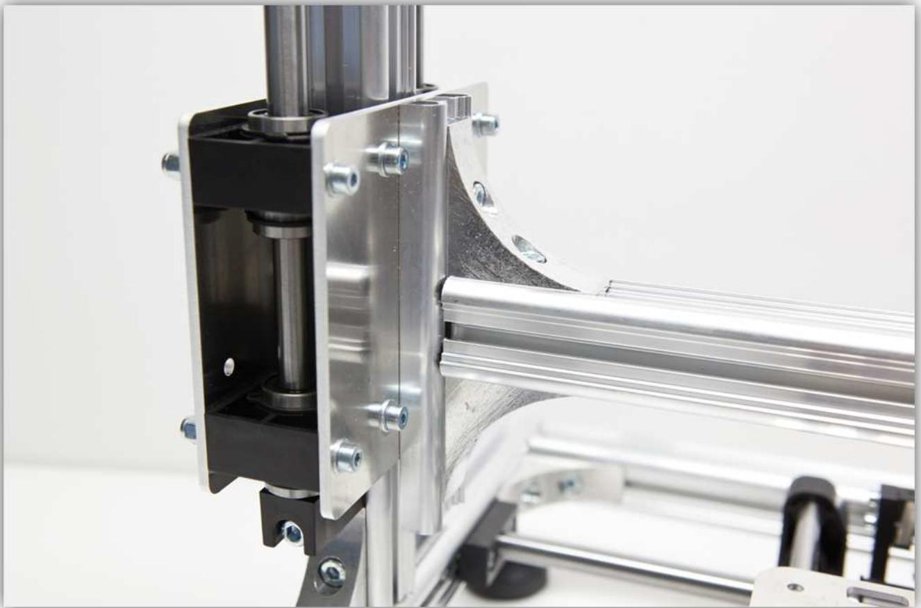
Make sure there is about 5 mm of a gap from the top of the Z CARRIAGE and the top of the ANGULAR MOUNT.
