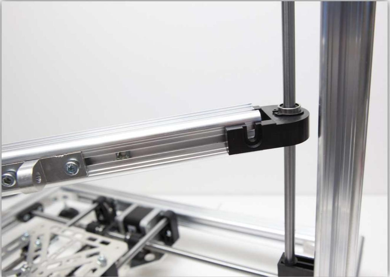
Now slide the two ANGULAR MOUNTS into the Z CARRIAGE. Be careful that while doing this, none of the square M5 nuts slide out of the angular profile.
