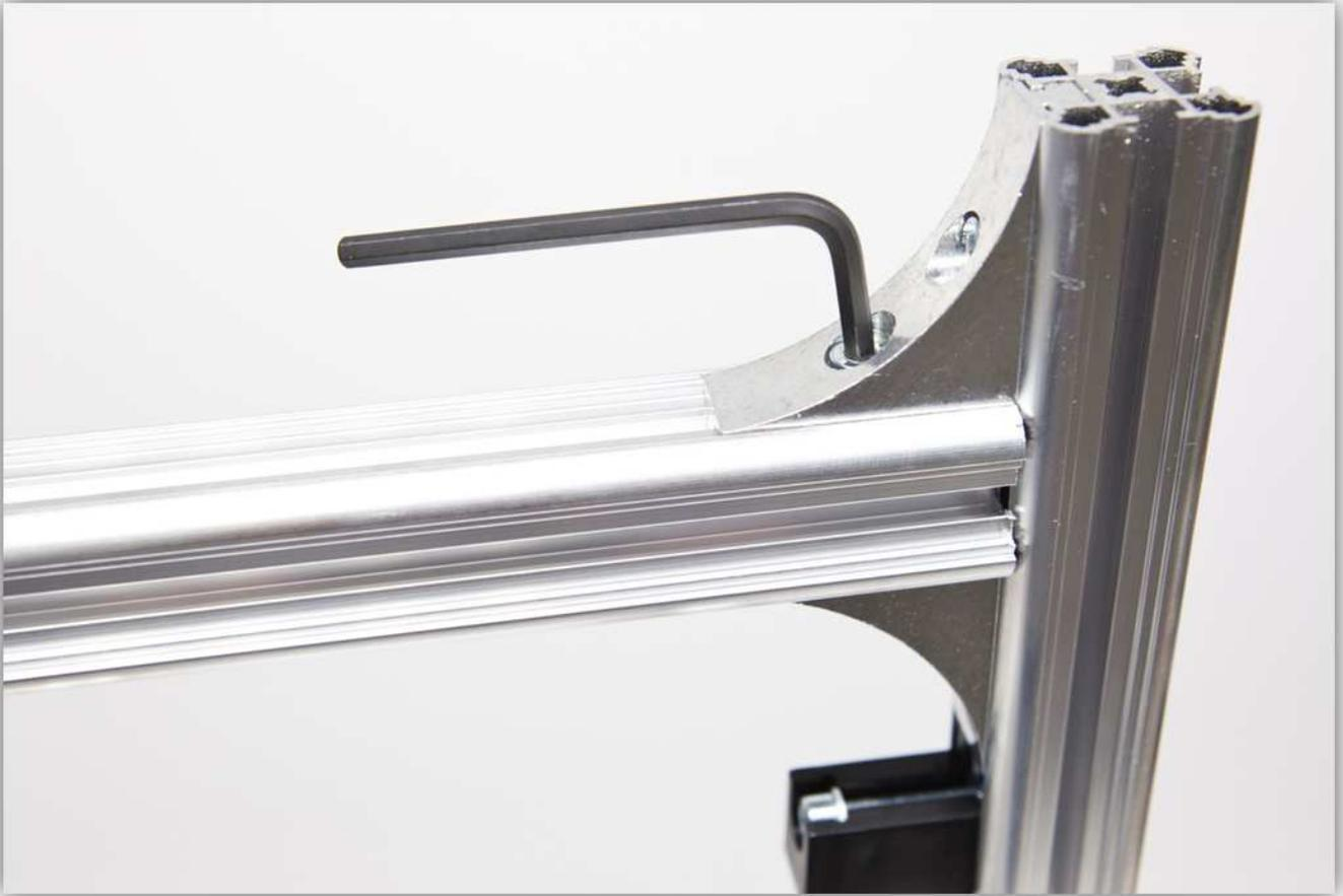
Slide the two square nuts on the opposite of each other in the extruder arm towards the BEARING CLAMP Z SMALL piece.
