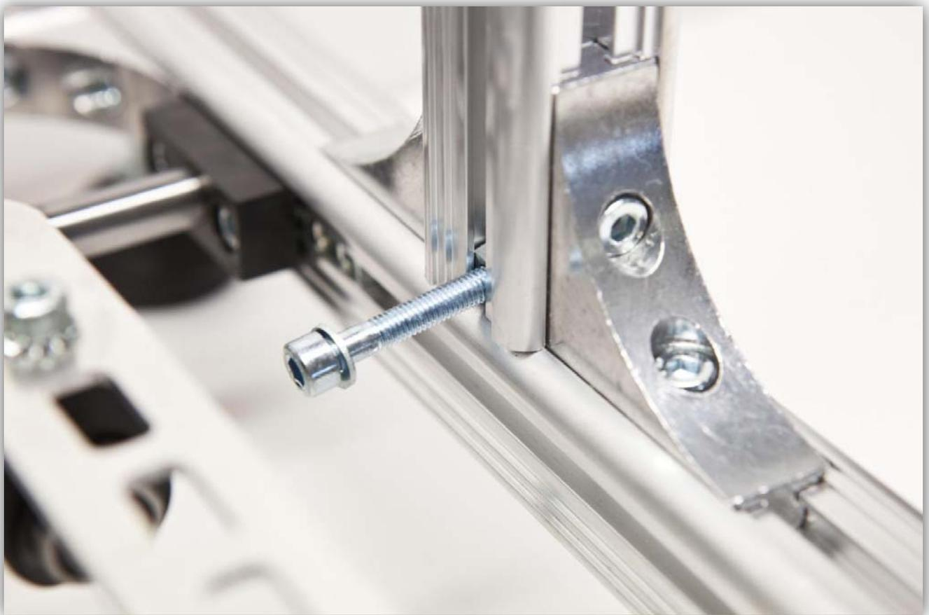
Slide one of the ROD CLAMP Z SMALL pieces over this bolt and make sure you tighten this bolt so that this piece sits at about 6 cm (2.36") of the base frame.
