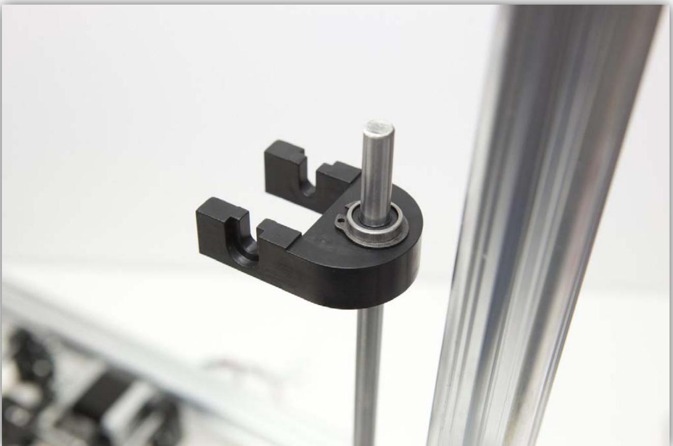
Slide one of the M5 bolts (with washer and square nut) and slide it down the ALUMINIUM PROFILE and slide a ROD CLAMP Z SMALL over this bolt. It should fit over the rod.
