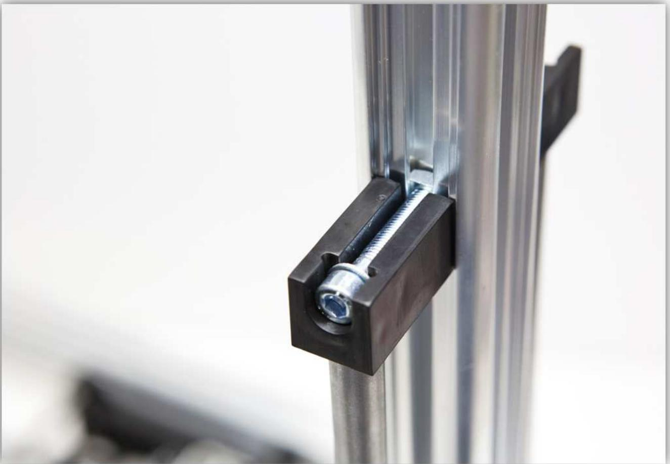
Tighten these bolts. **Do not over tighten.**
