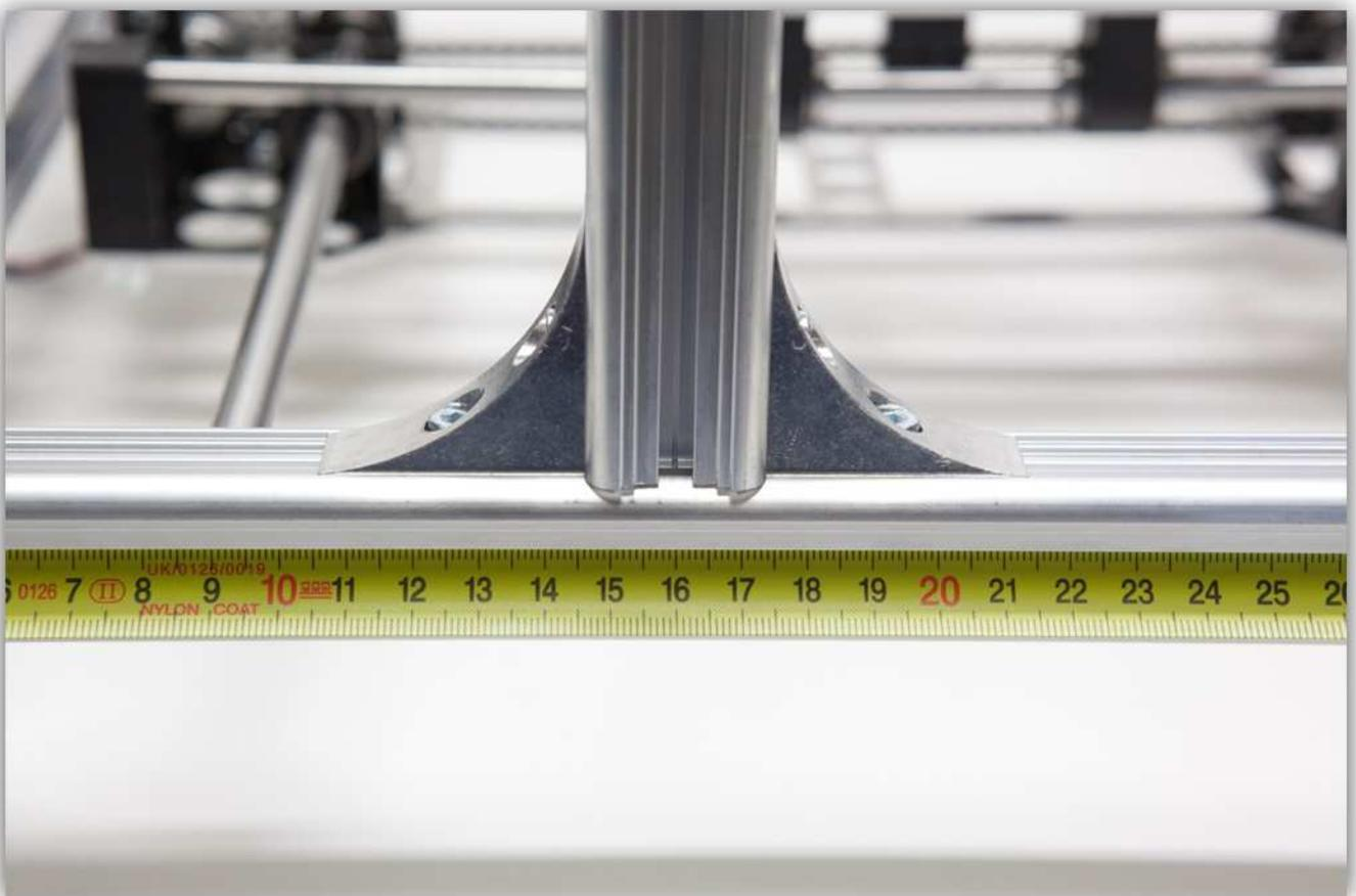
Tighten the bolts on the ANGULAR MOUNTS.
