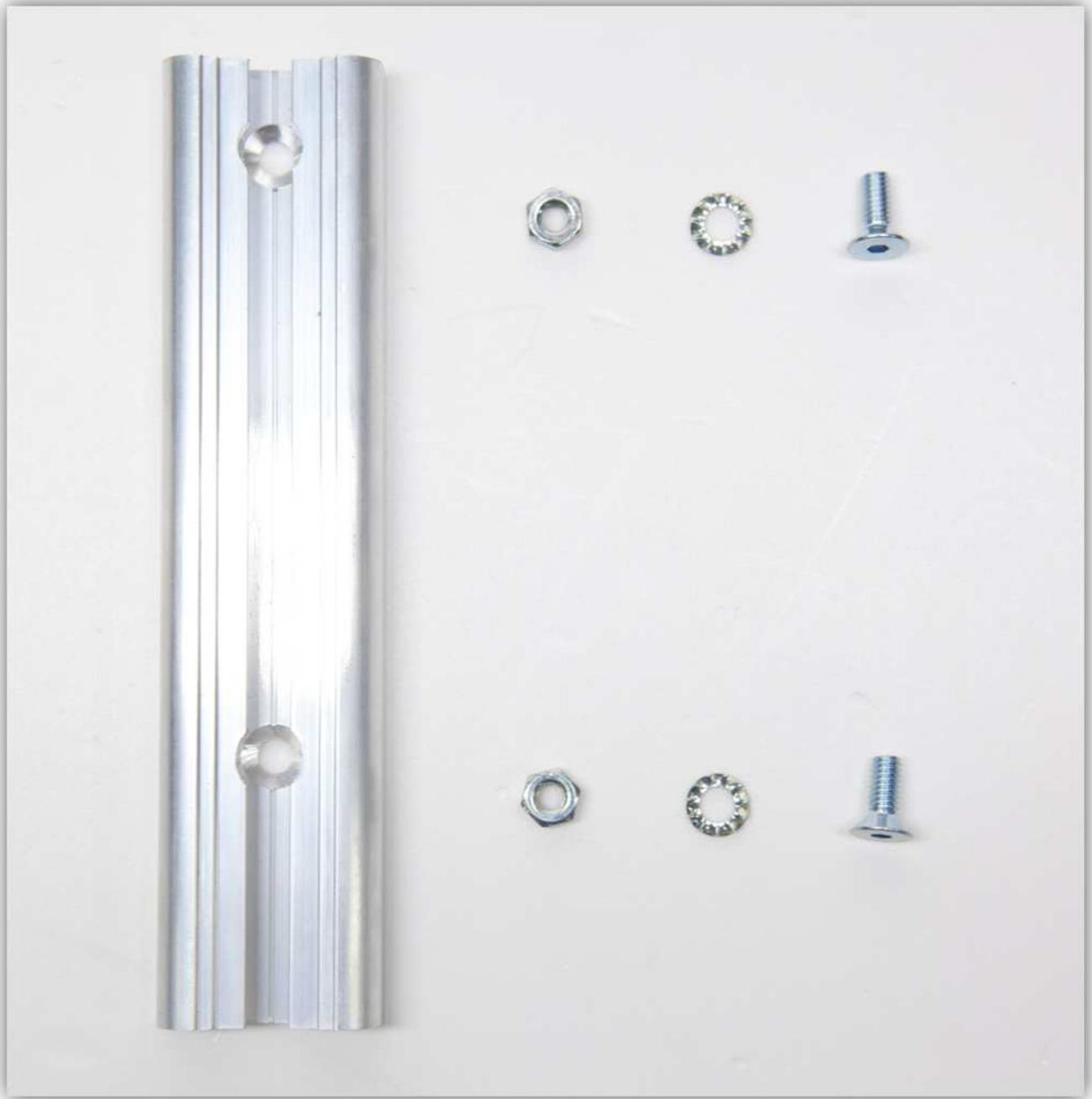
Use the 2 M4 countersunk screws to attach the small ALUMINIUM PROFILE to the Z CARRIAGE FRONT piece.
