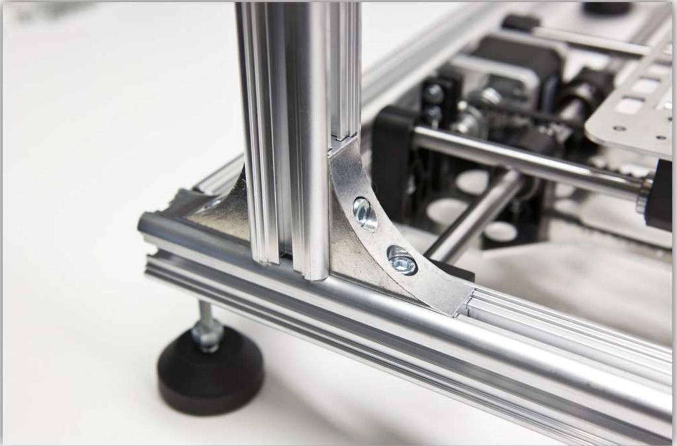
Slide it further down the profile until its centre is at 16 cm (6.3") from the edge of the base frame.
