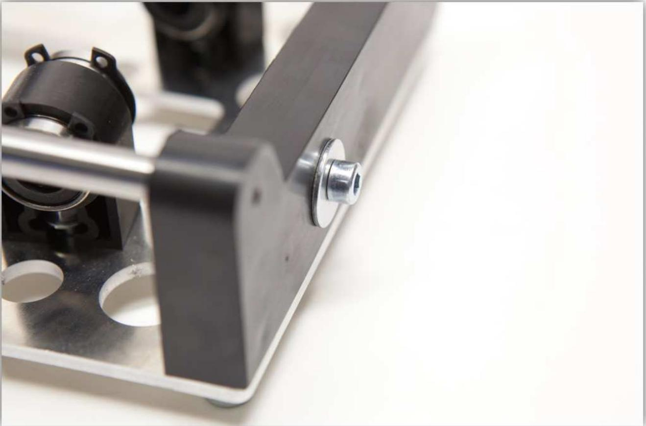
And the small M5 washer and an M5 locking nut on the other end. **Do not tighten the locking nut. Just put it on so it won't fall off. We will come back to this part in a few steps.**
