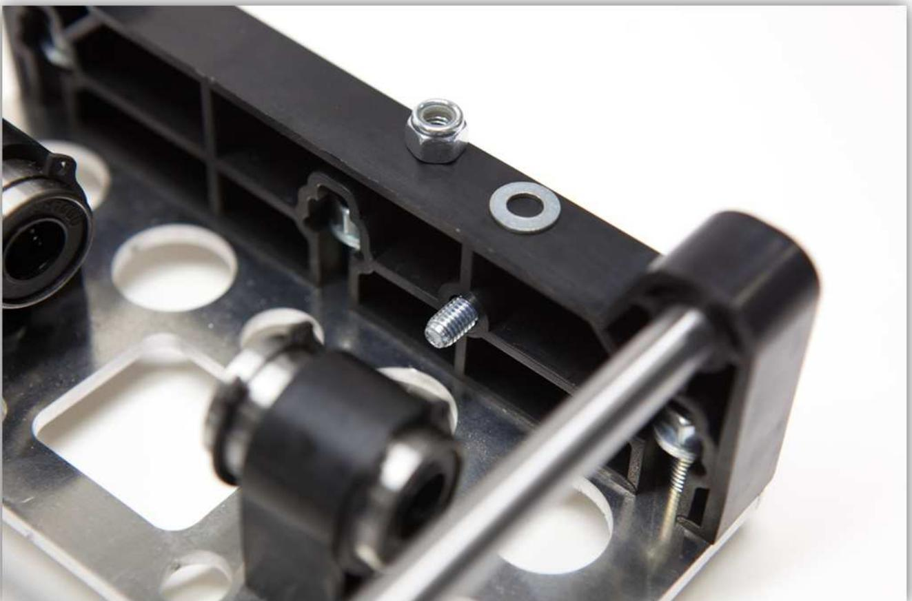
Place the small aluminium bracket as shown in the picture and tighten the assembly.
