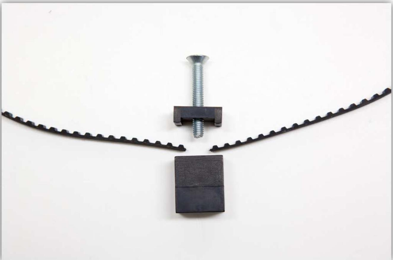
Assemble them as shown in the picture. **Take notice that the belt sits between the clamps exactly as in the picture.**
