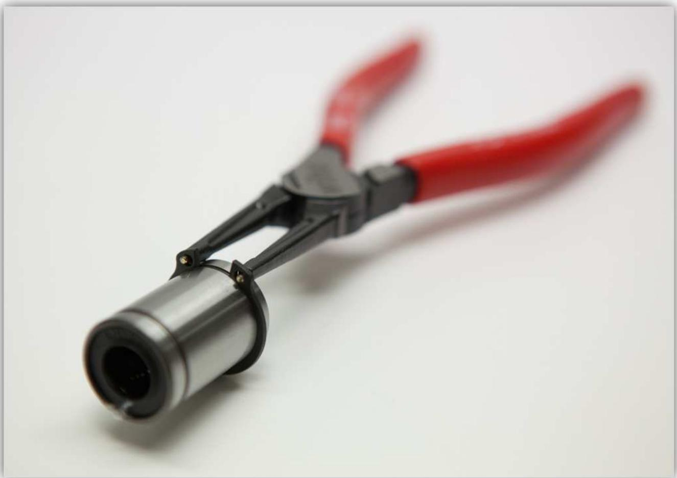
Slide the bearing with one circlip inside one of the BEARING CLAMP X pieces:
