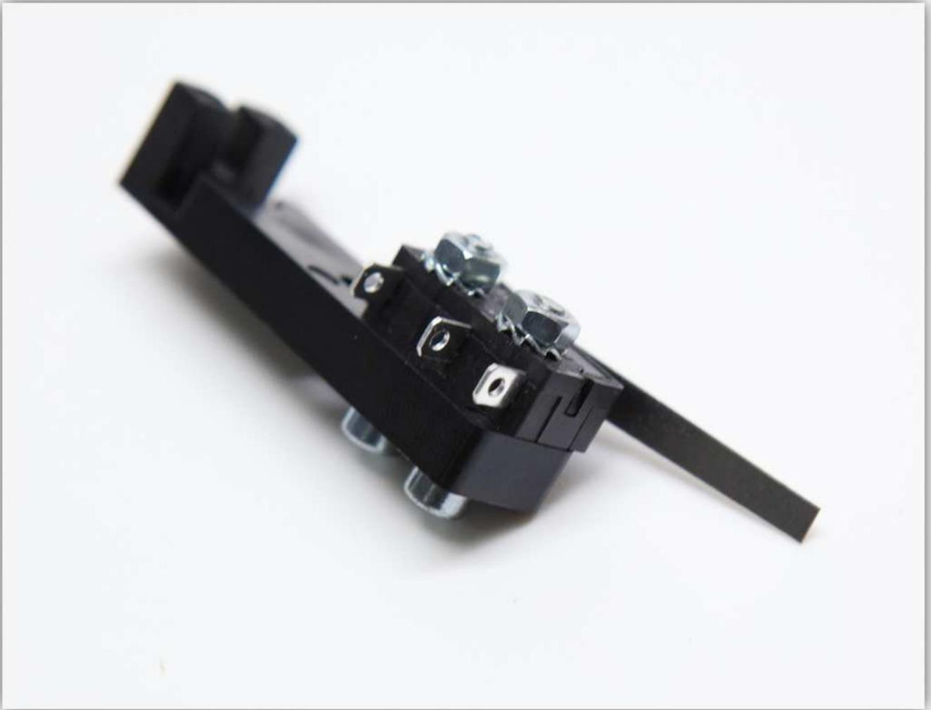
Cut 10 mm (0.39") of the lever of the micro switch, be careful not to cut too much.
