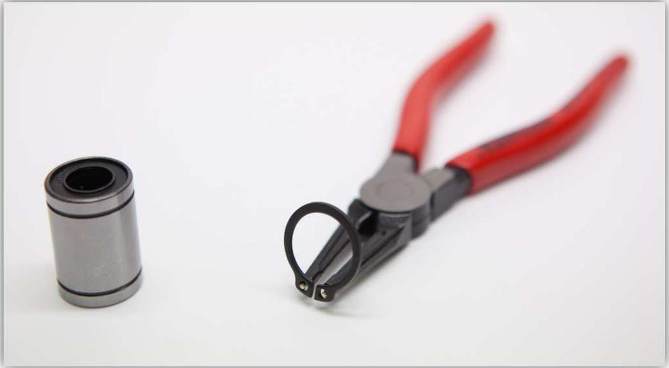
Use the circlip pliers to carefully fit the circlip around the LM10UU linear bearing.
