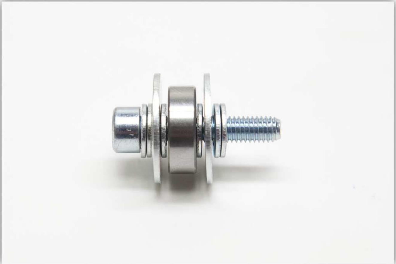
Use an M5 locking nut and an M5 washer and mount the assembly as shown in the picture. **Do not tighten this assembly.**
